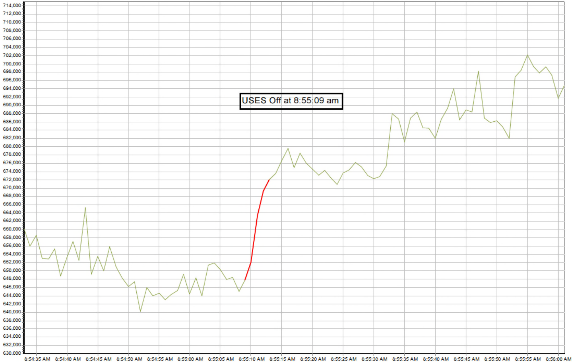
Graph 1A Above is the instant change in Real Power Demand in watts during the TIS testing on February 22, 2013 at 8:55:09 am, with 11 USES ® model XL-3D-480V and 1 USES ® model XL-3Y-480V power conditioners operating. The real power demand is instantly reduced 24.285 kW in low load conditions.
